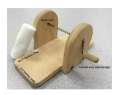
A simple bandage rolling "machine" can be created from scrap wood and a wire coat hanger:
